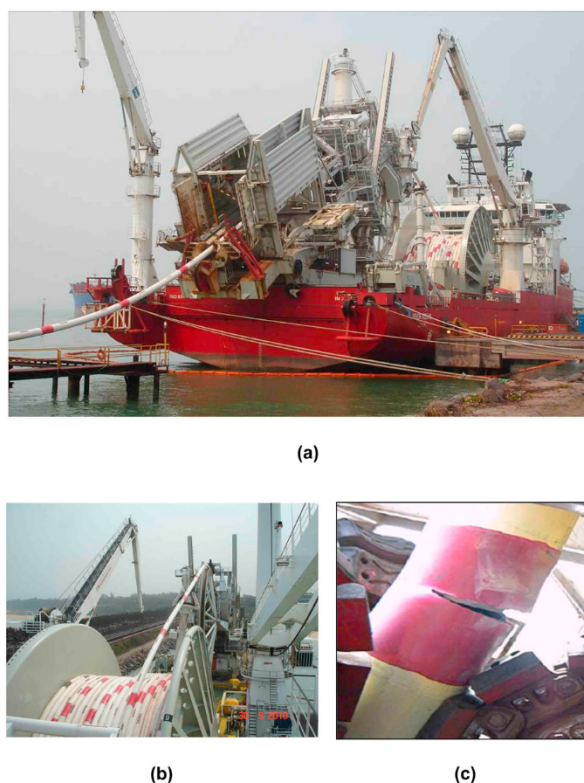
Fig. 1. (a) Reeled pipe lay vessel with a main deck-mounted storage and deployment reel; (b) View of pipe reeling onto the drum; (c) Pipe failure from an undetected flaws at the girth weld (Pictures courtesy of A. Garmbis (2012)).
